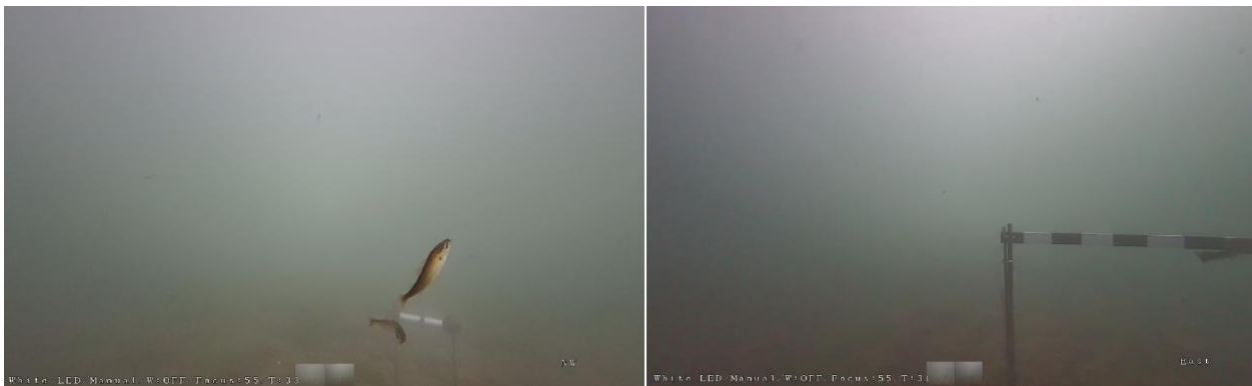
Figure 8: A view from two different cameras after reflective (left) and standard contrast (right) targets were installed as part of the HydroAware project.
