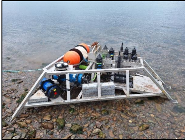
Figure 7: FAST-2 platform equipped with five Innovasea acoustic receiver technologies (with duplicates for redundancy), an ADCP and hydrophone for recording flow speed and underwater noise.
